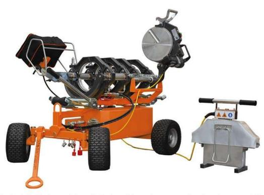
Self-aligning hydraulic butt fusion machine, suitable for welding underpressure pipes for water, gas and other fluids up to Ø 8" DIPS (250 mm). Built according to the International standards ISO 21307 HIGH PRESSURE (the clamps cylinders work with a pressure range that is three times and a half higher than the ISO Low Pressure ones. This enhances productivity, with a welding time saving of 60%). DELTA 250 TRAILER includes:
